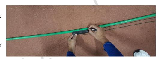
4) We can use any material we want to make the bow grip... I use thermal shrink tube that used in electrical works and it's easy to find it. I use a lighter to shrink it and in no time I got a grip. You can use rope or any other material you want.
