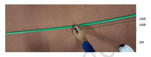
3) The mark in the center of the tube is the center of the grip so we measure 5cm left and right of the mark and put 2 new marks in order to have the place of the bow grip marked ...
